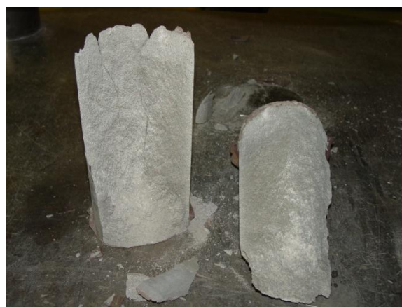
Grout cylinder after compression test
