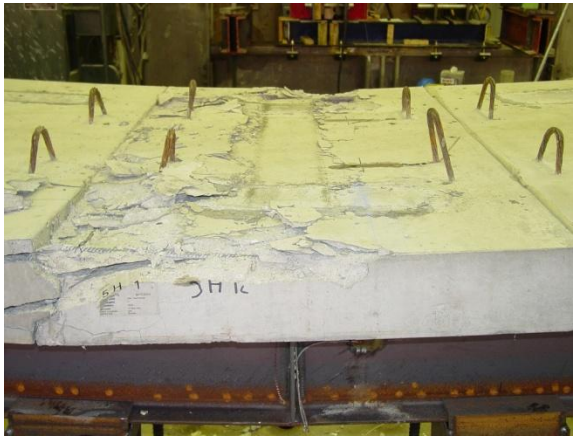
Yield of bottom flange and concrete crushing at load point section
