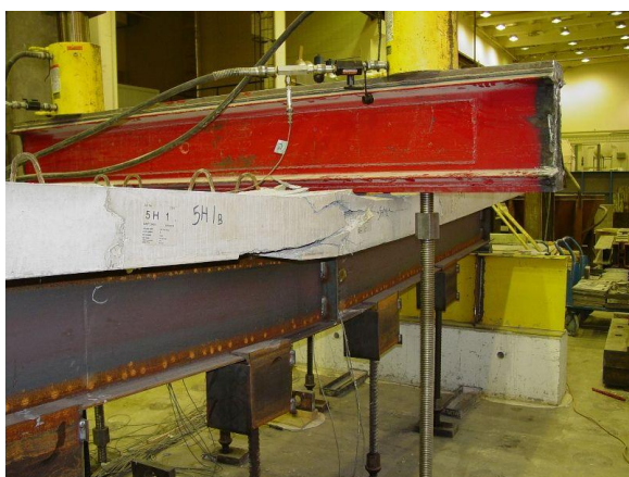
Concrete crush at west mid-span (south)
