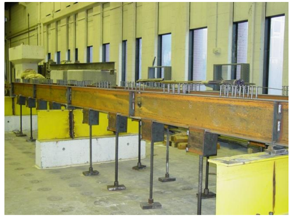
Girder placed over bearing/supporting beams
