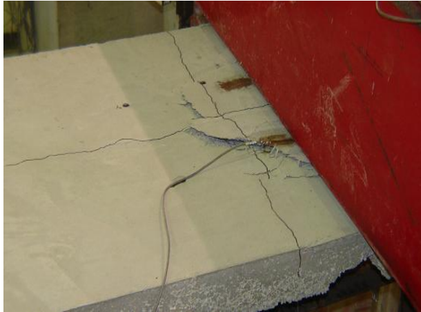
a) Crushing the concrete slab at the point load
