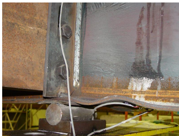
Close-up flange buckling (south girder)
