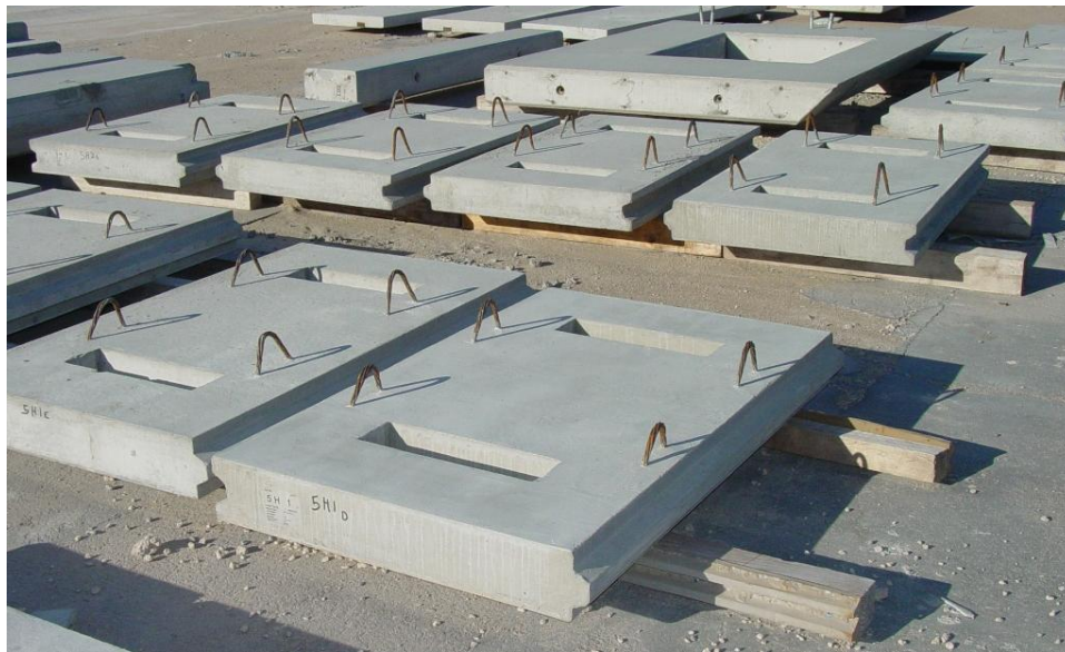
Figure 4-11. Precast concrete deck panel at Concrete Industries Inc yard.
