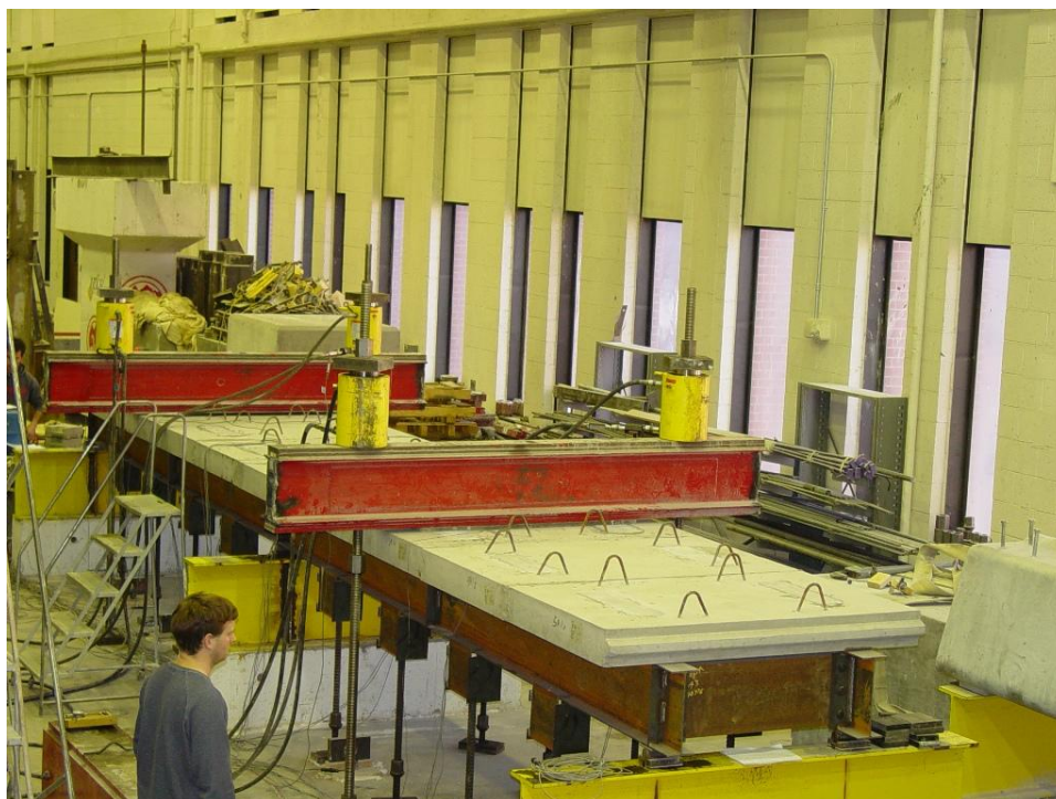
Figure 3-36. Ultimate load test setup.
