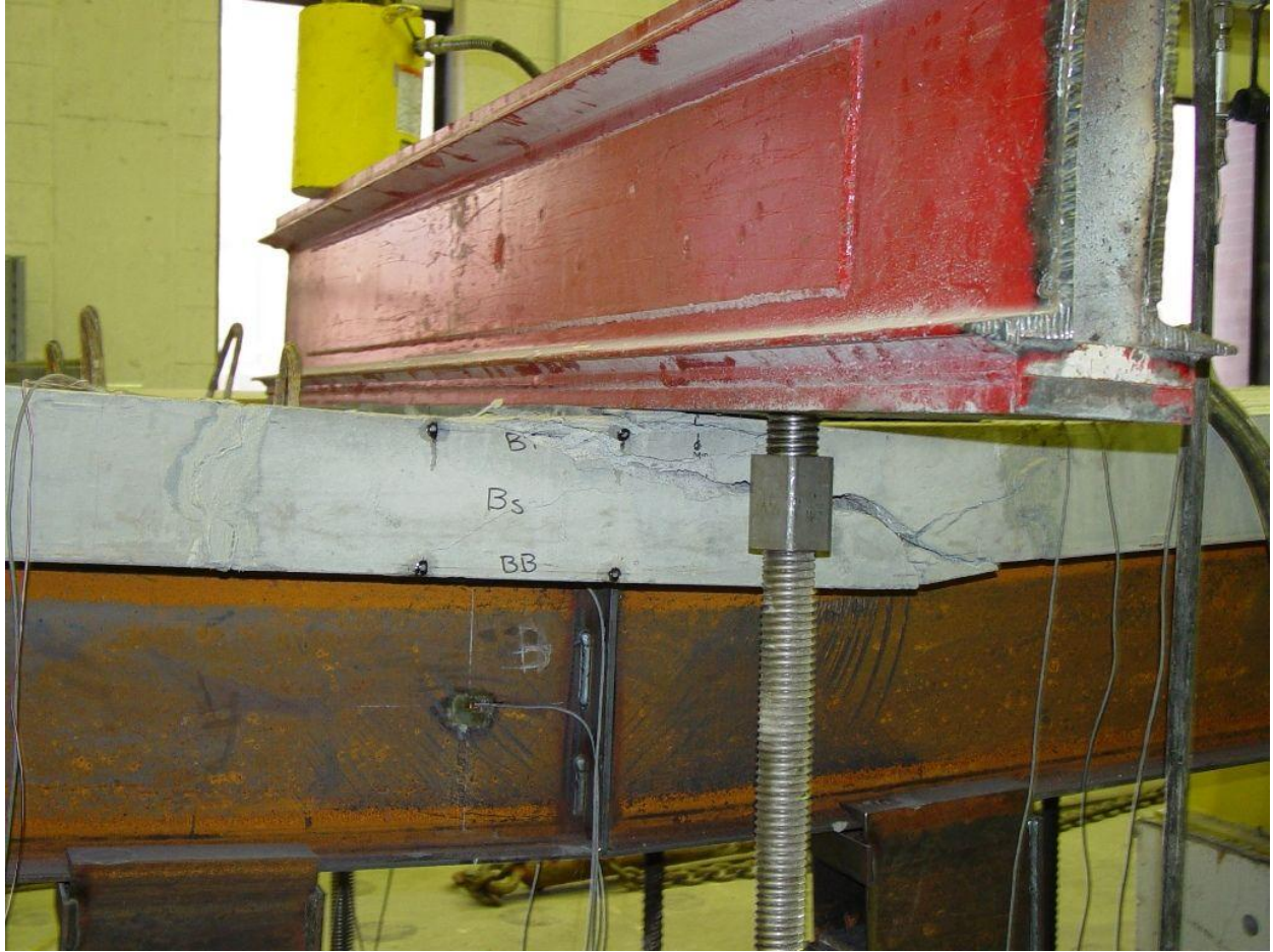
Figure 4-34. Concrete crushing under the loading location at mid-span (west side).
