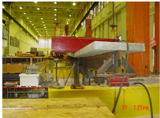
b) Large deflection (yielding/buckling) failure mode
