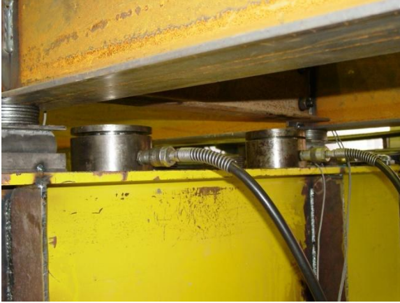
Pancake jacks used to shim the system
