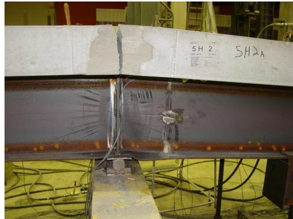
Web/flange buckling and large crack width over center support section
