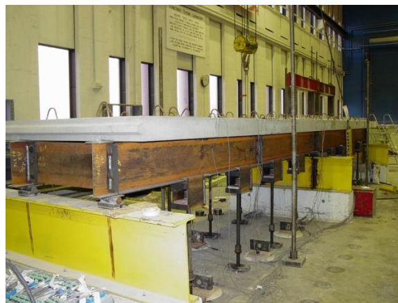
Monitoring concrete creep
