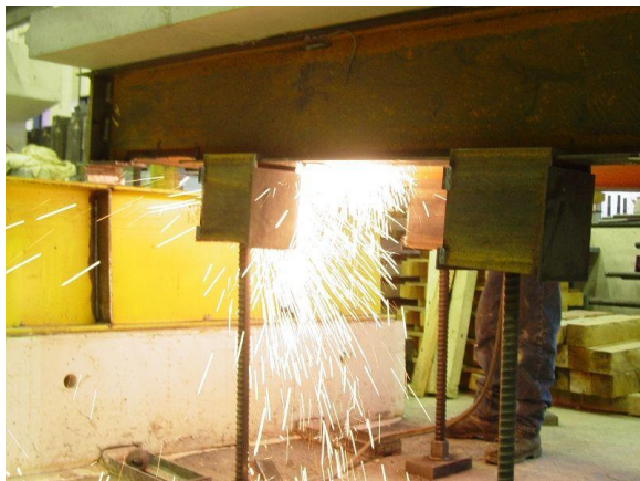
Steel sample removal
